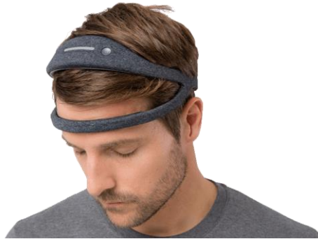
Figure 1. Dreem headband worn during four nights by the participants in the field study. The headband measures frontal and occipital brain activity (EEG).
