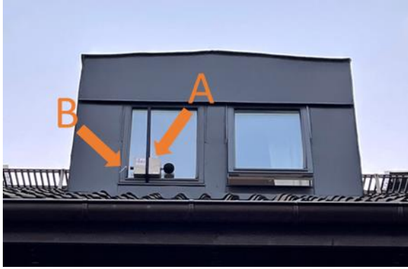
Figure 1 Typical mounting of outdoor sound level meter. A: Sound level meter. B: power cable passing through window gap while window fully closed.
