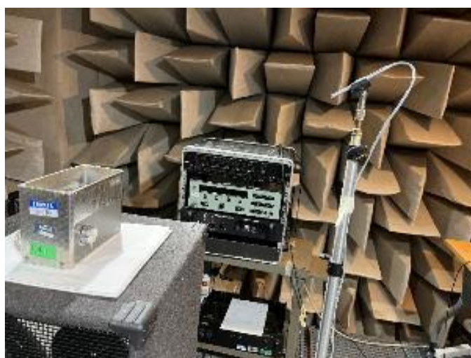
Figure 1 – Measurement set up. The configuration shown is \theta = 45^\circ , \phi = 0^\circ
