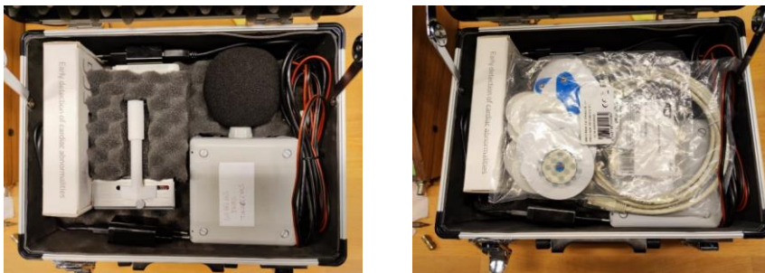
Figure 6: The measurement box: eFaros 90, Tinkerboard, wireless microphone), at the right the box including the consumables (electrodes, spare cables etc.).
