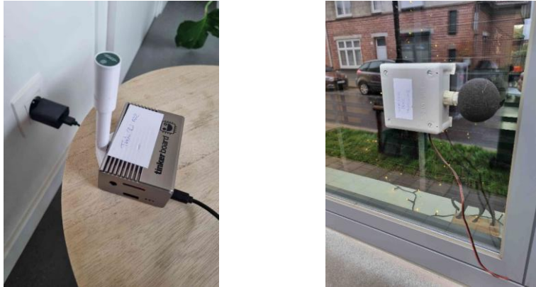
Figure 2: The indoor noise unit (left) and outdoor noise unit in an operational setting.
