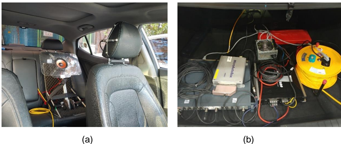
Fig.4 Equipment for active noise cancellation of cavity noise (a) error microphone and speaker for 2nd sound source (b) Auto box controller, lowpass filter and speaker amplifier.
