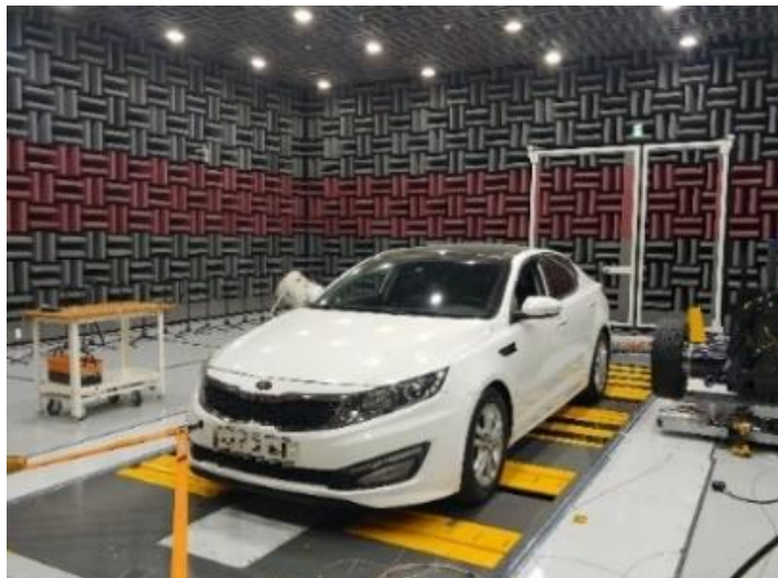
Fig.2 Test car excited by impact bar on roller of chassis dynamometer.
