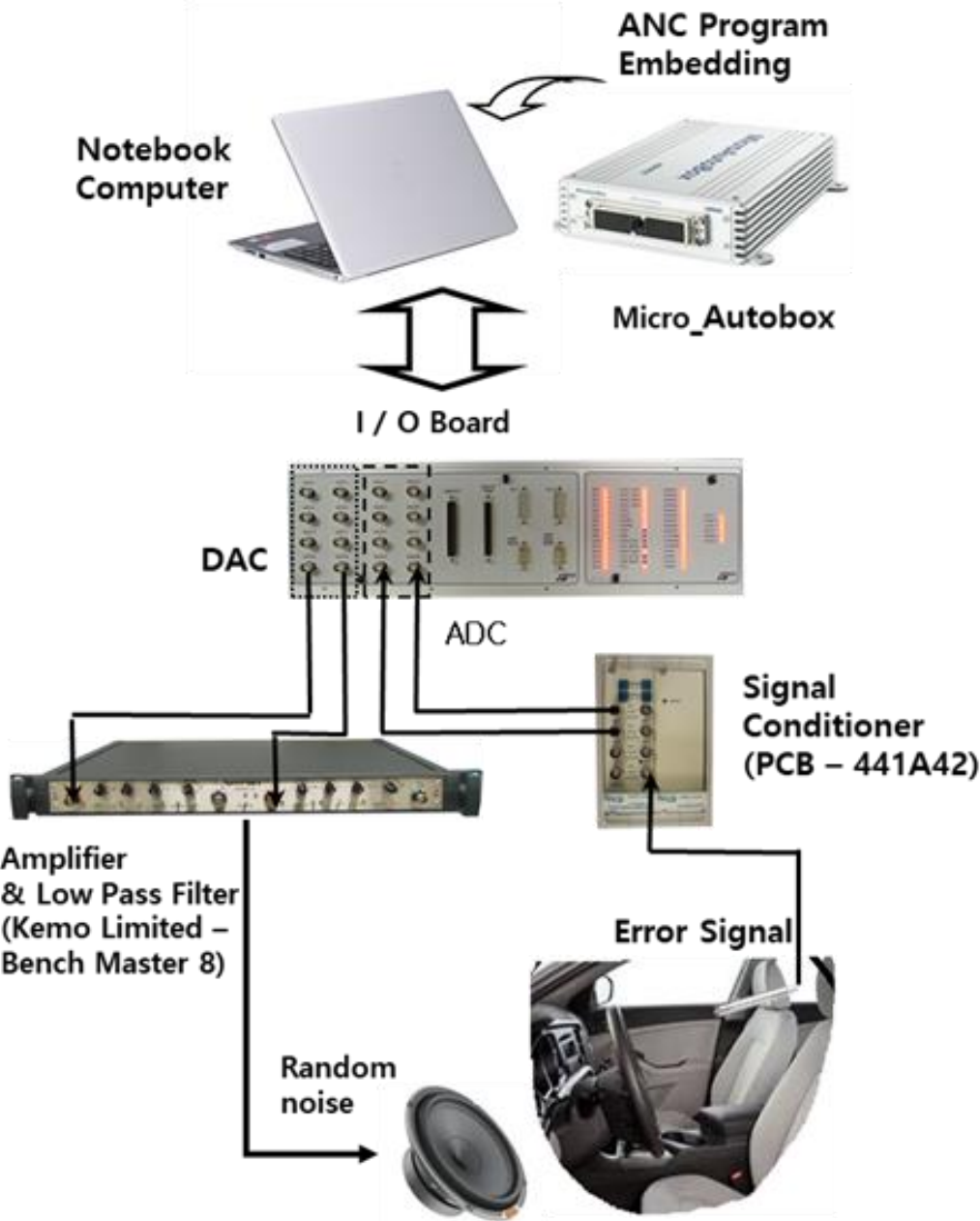
Fig. 5 Equipment and data flow used for transfer function of secondary path.
